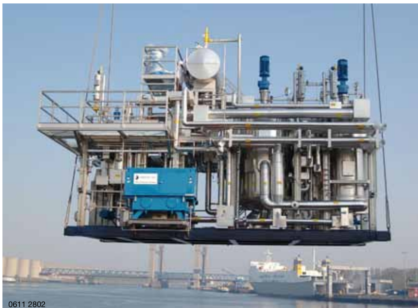
0611 2802 Skid mounted suspension crystallization plant for MDI
